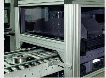
Break discs run through the inspection housing on a roller belt.
