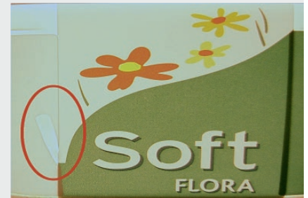
Error at welding areas, overlapping and displacement are detected reliably.
